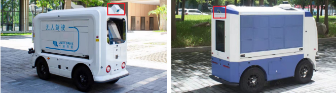
Fig. 2. LiDARs are installed towards ground
